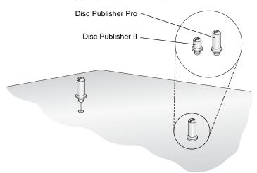
• Attach the stand to the unit using the adjustment bolts and the washers. **Do not tighten the bolts at this point!**
